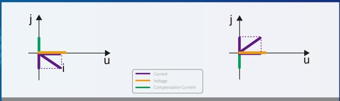
Because most of the electrical equipment is inductive load, the power factor is obviously less than 1 during operation, a large amount of reactive power needs to be taken from the grid. Therefore, in order to improve the power factor of the grid, it must compensate the reactive power in the grid.
